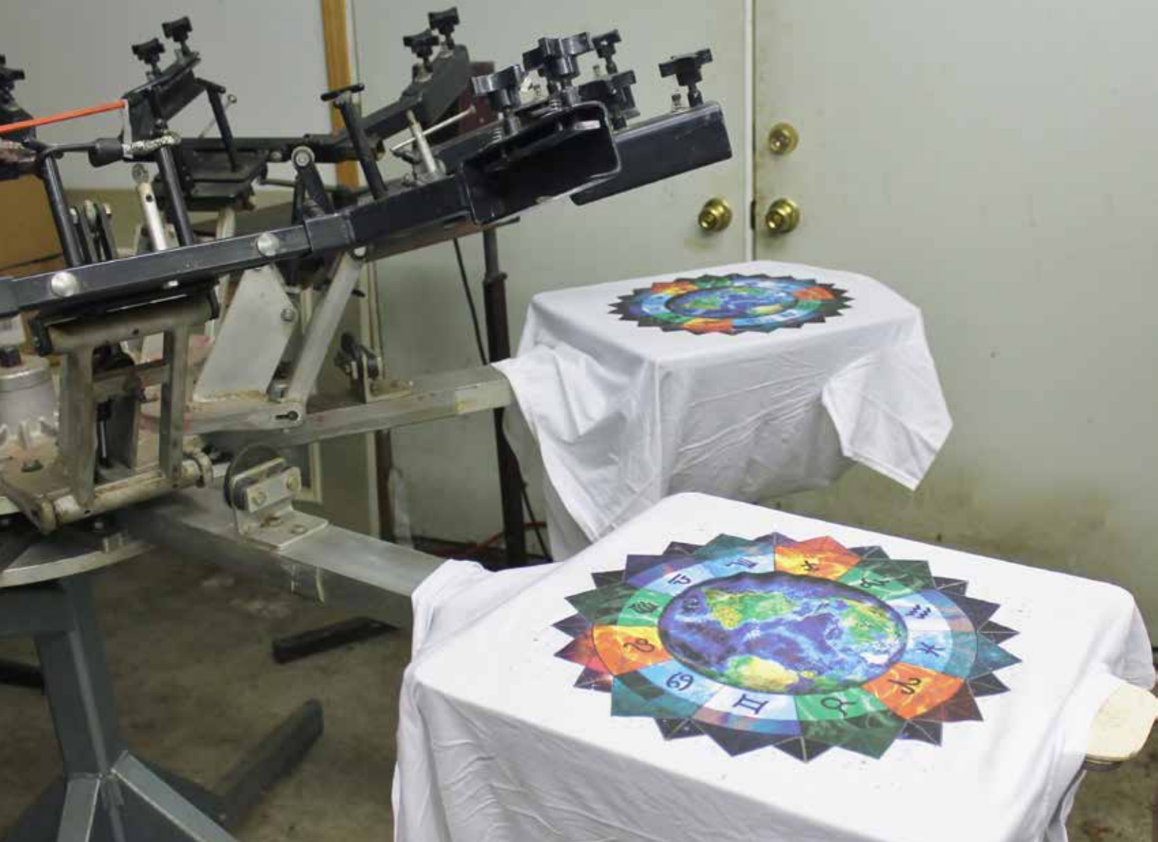
Shirts printed with Aquarius Soft Base CMYK, showing the ability to capture a wide spectrum of color with just four screens plus a white highlight screen. Credit: Jenny Ortolani.
