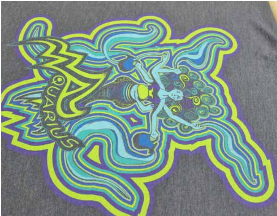
Three-color psychedelic design printed with Aquarius Bright Discharge Base ZF. All discharge colors are printed with 200 mesh and one squeegee pass for each color. Credit: Jenny Ortolani.
